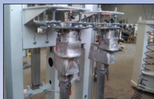
FORME INTERCAMBIABILI INTERCHANGEABLE HEADS AND BUCKS
